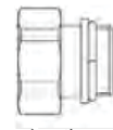
Fig 1.1 showing the captive nut to link the mixing unit to the manifold
