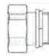
Fig 1.1 showing the captive nut to link the mixing unit to the manifold
